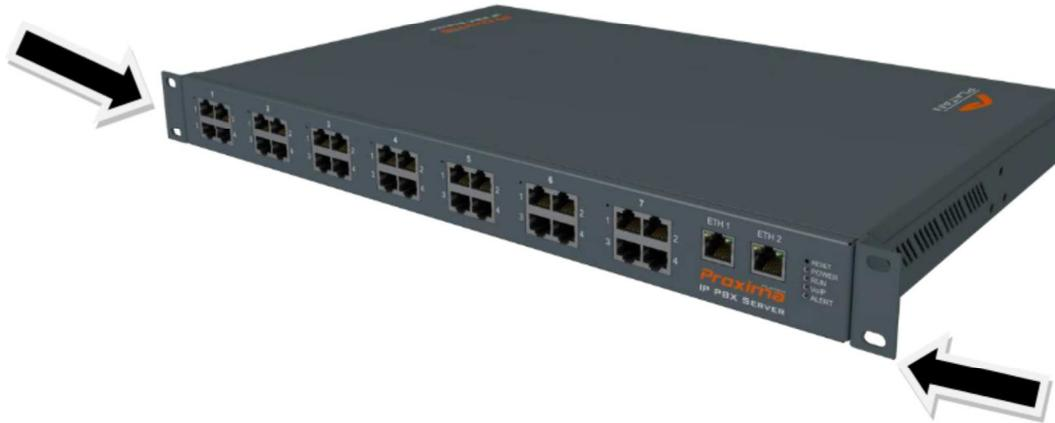
2. Install the CLIPKO mounting catches in the RACK 19” cabinet buses – 1U spacing (1 mounting hole counting from the mounting bus U size multiplication marker should be left empty – the markers are indicated in the figure by arrows).
